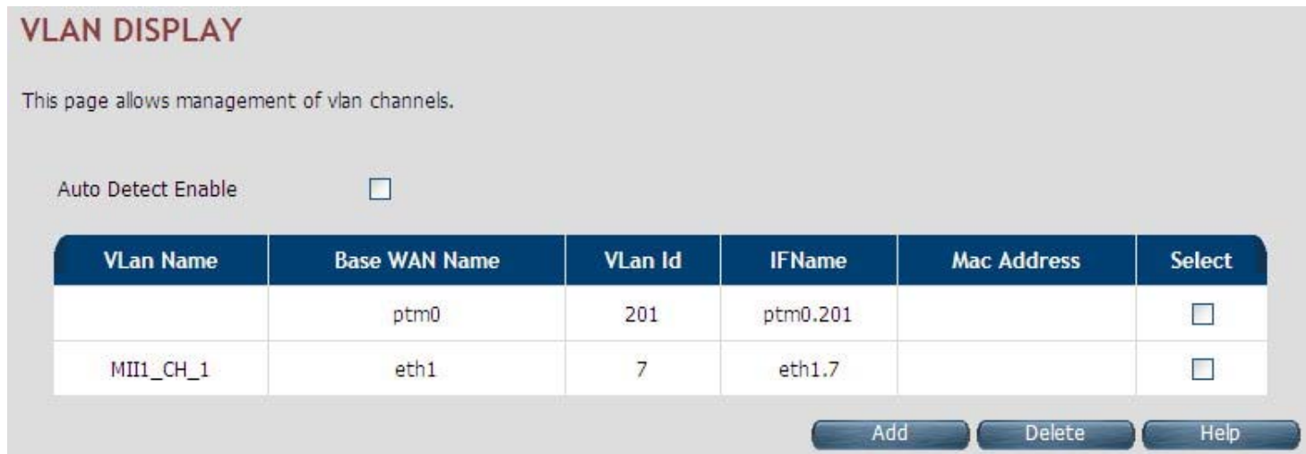
Figure 4.6.4.1 VLAN Channel Configuration Display (Auto Detecting does not check the checkbox)
